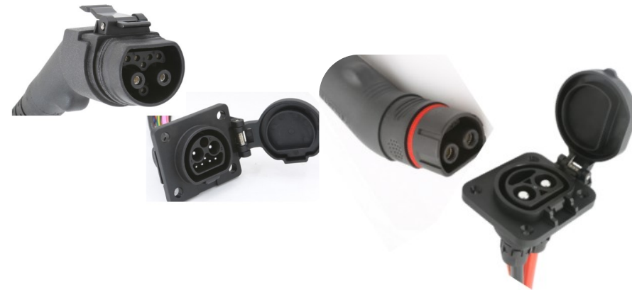
HG01/02 2+6P 20A /80A Charging Plug and Charging Port on the vehicle
