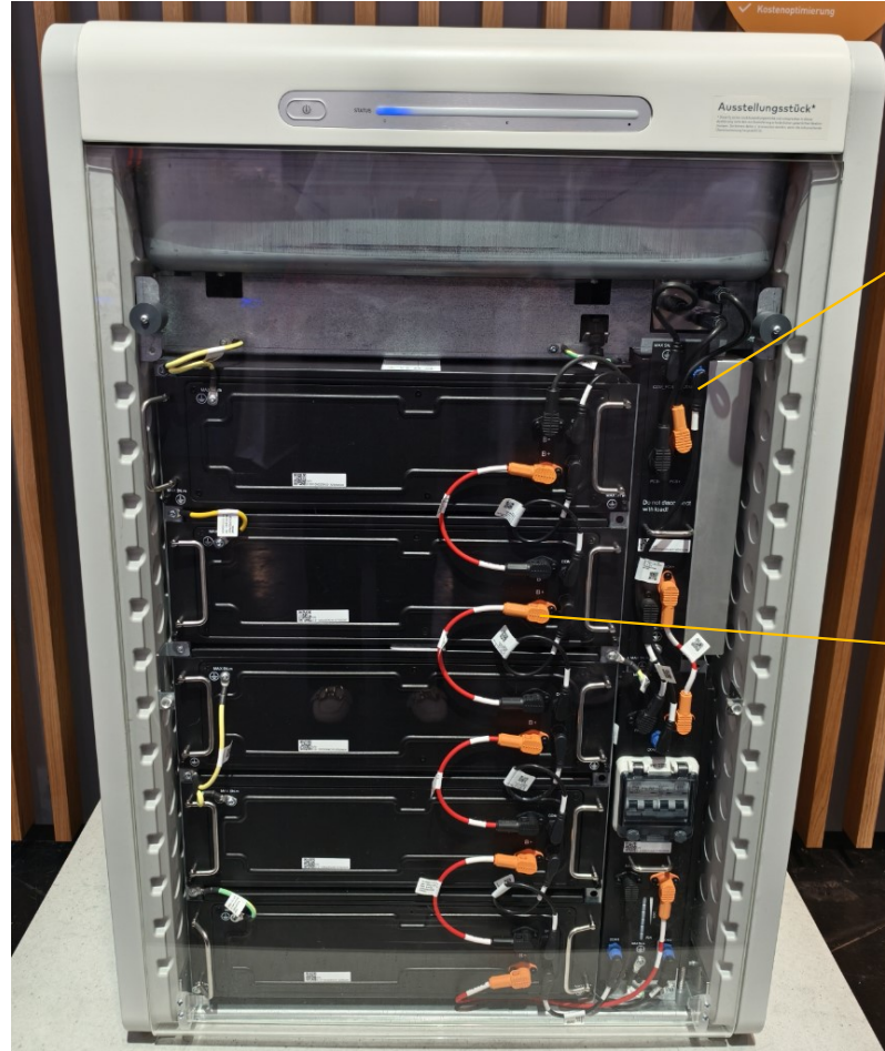
CPL Single Pole for Power Transmission (120A)
